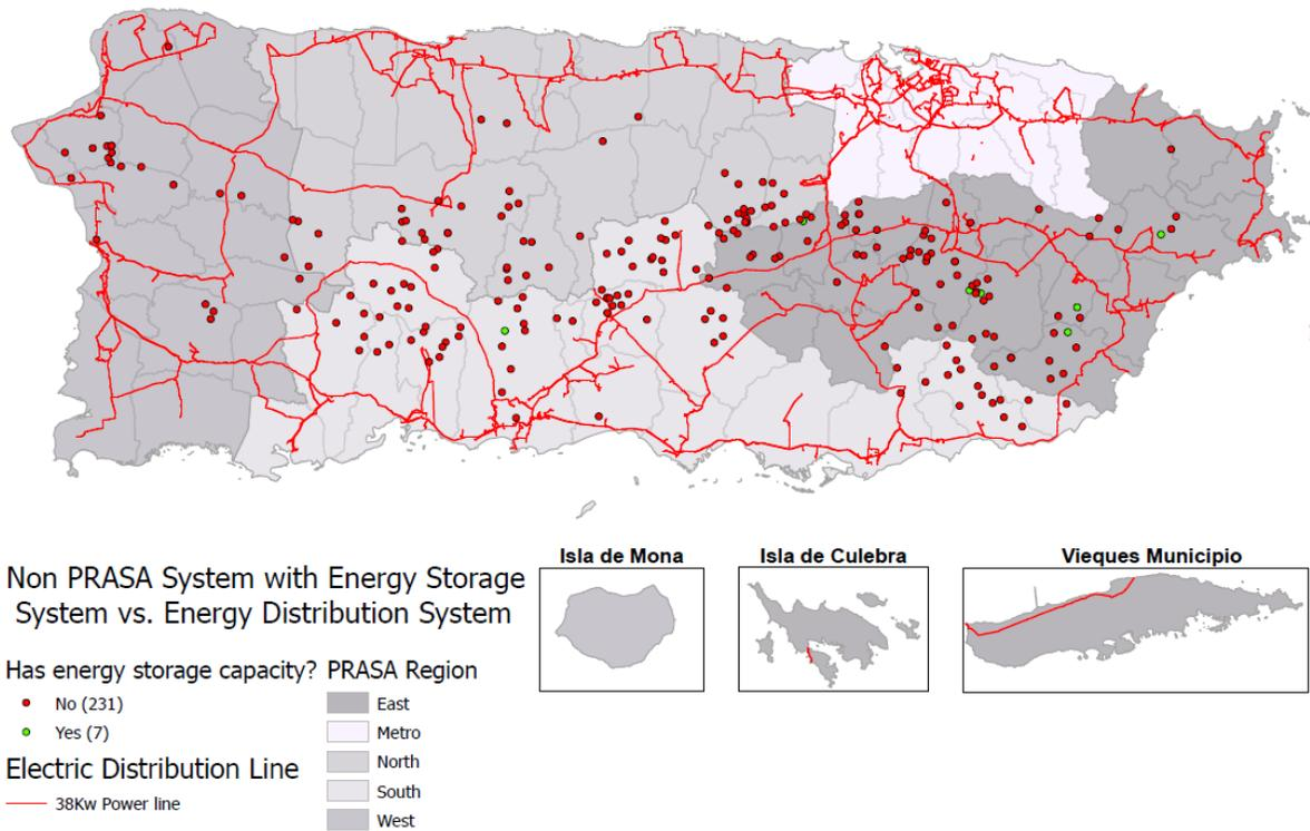
Figure 38 - Non-PRASA System with Energy Storage
